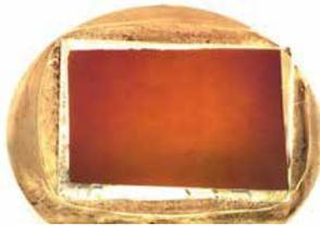
Thin semiconductor or other substrates to less than 200 nm to enable backside SIMS analysis.
